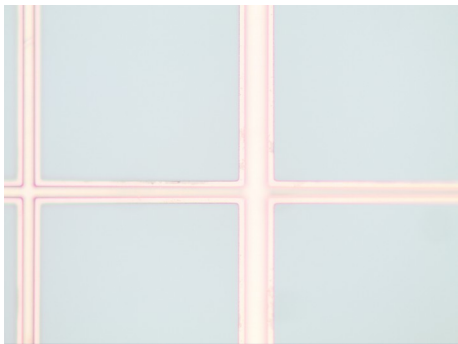
Regular bar grid at junction of thicker center bar
